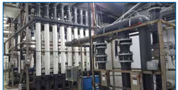
Two skids each using twenty X-Flow Membrane Elements (image courtesy of BioprocessH2O).
