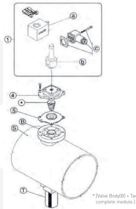
\* [Valve Body(B] + Tank(S) + Valve blowpipe (T) are to be considered single and complete module.] (No spare parts available for this configuration.)
