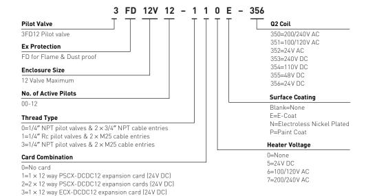
$4=2 \times 12$  way ECX-DCDC12 expansion cards (24V DC)  $5=1 \times 12$  way ECX-ACAC12 expansion card (100-240V AC)  $6=2 \times 12$  way ECX-ACAC12 expansion cards (100-240V AC) 7=1 × PSCX-DCDC12 expansion card + 1 × Hub (24V DC)
