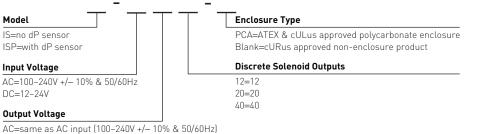
AC=same as AC input (100-240V +/- 10% & 50/60Hz) LAC=24V 50/60 Hz (AC input only). DC=same as DC input (12-24V DC),
