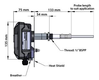
PROBE ROD LENGTH 300mm | 600mm | 1000mm
