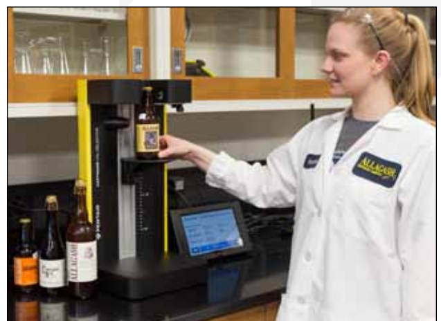
Heather Muzzy, a Quality Control Specialist at Allagash, tests the CO 2 level in a bottle of Allagash's signature White with Haffman's non-invasive CO 2 -Selector.
