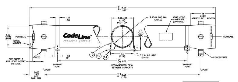
VIEW AT CENTER SUPPORT CENTER VESSEL ON 2 OR 3 SUPPORTS AT SPAN(S) "S" : 3 SUPPORTS REQUIRED FOR LENGTHS -4 AND OVER
